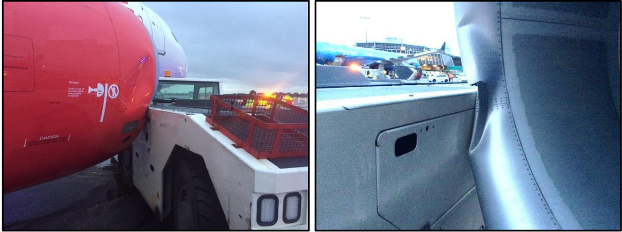
Photo Nos. 1 & 2: Damage to starboard engine cowling
